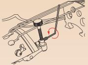
Making sure that the string hook moves smoothly, carefully turn the adjustment screw with a hex wrench, clamping the adjuster in place.
