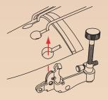
Insert the string hook section of the violin adjuster into the tailpiece hole from below.
