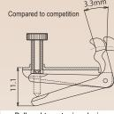
Ball-end type tuning device Weight = 5.2g
