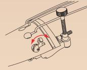
2 Slide the string hook section from the tailpiece hole towards and partially into the string guide hole.
