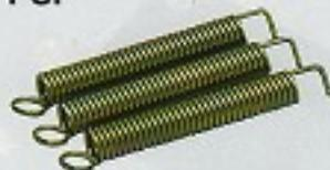
Vibrato bridge is balanced by string tension and coil springs used for pulling its block and it is only by the power of coil springs to return to the original position after dive bombing of vibrato arm. It is important to have durable spring for all kinds of vibrato bridge and PSP power spring minimizes tuning instability by its durability when using vibrato.
